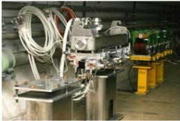
The LHC collimation system (over 150 individual collimators are situated around the LHC ring) protects the accelerator against such beam loss; which would otherwise impinge the supramagnets and cause them to fail ("go critical"). http://lhc-collimation-project.web.cern.ch/lhc-collimation-project/
