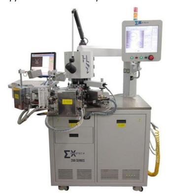
The manufacture of modern electronic equipment (mobiles, consumer, white goods and industrial electronics) requires many millions of individual electronic SMD components (resistors, capacitors, diodes, transistors etc.) every day. Each of these parts must be individually tested, before it is assembled onto a PC-board.
