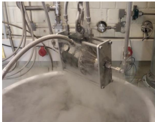
Figure 4. OCV- Campaign test at LN2 temperature conditions (77 K) [6]
