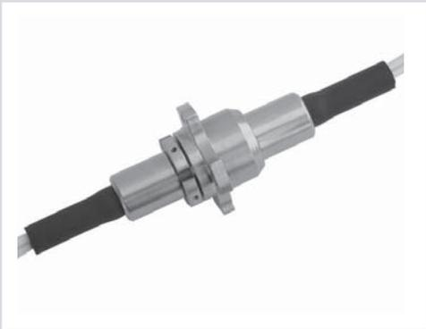
This dual-pass Fiber Optic Rotary Joint (FORJ) connects two independent fiber channels simultaneously. It allows uninterrupted transmission of optical signals while rotating along the common mechanical axis. It is designed to accommodate at least one multimode fiber. The other channel can be either single or multimode fiber. Princetel's unique design has raised the standard for size and performance of two-channel FORJs.
