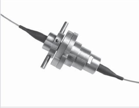
The MJP series FORJs are designed to accommodate specialty fibers such as large core or plastic fibers. The device is free of index-matching fluid and therefore is ideal for spectroscopic applications. Stainless steel construction and ceramic ball bearings make the device rugged, precise, stable, and long lasting.
