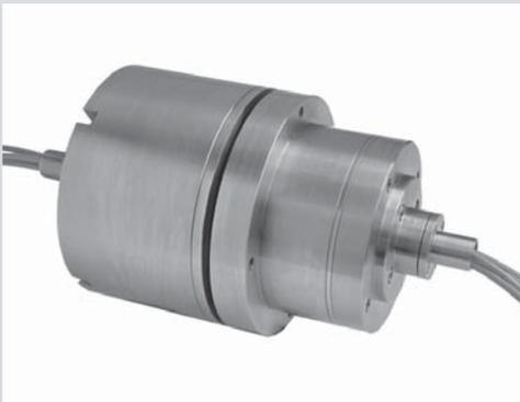
Multi-pass Fiber Optic Rotary Joints (FORJs) connect 2-10 independent fiber channels simultaneously. They allow uninterrupted transmission of optical signals while rotating along the common mechanical axis. The RJ<sub>n</sub> series FORJs feature extremely low crosstalk performance (<-50 dB) for singlemode and multimode fibers. All channels can accommodate either singlemode or multimode fibers. It is also possible to combine the two types of fibers in one device.
