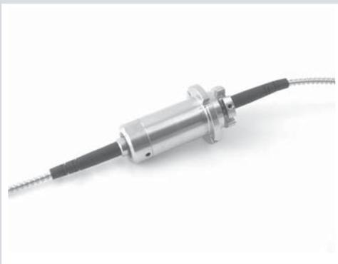
Model RPC series FORJs are designed to offer extreme pressure rating of 20,000 psi while maintaining identical optical performance as the RPT series. 900 um Hytel tight buffer and 2.9 mm armored jacket are standard cable arrangements.
