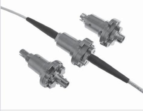
The R series Single-channel (SM or MM) rotary joints offer the most versatile designs on the market. The rugged body allows fiber pigtail, ST, or FC receptacles on either the rotor side or the stator side. One can configure the package to fit his need exactly. The standard base models are RPT, RFC, and FST for pigtails, FC/UPC, and ST/PC receptacles.
