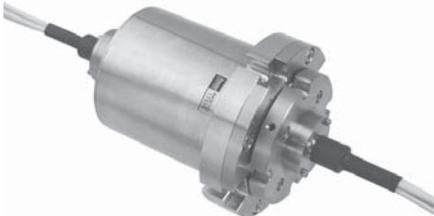
JX<sub>n</sub> series multi-pass Fiber Optic Rotary Joints (FORJs) connect 2-12 independent fiber channels simultaneously. They are almost identical to MJ<sub>n</sub> series FORJs except the location of the mounting flange. The JX<sub>n</sub> series FORJs feature extremely low crosstalk (<-50 dB) for single and multi-mode fibers. All channels can accommodate either singlemode or multimode fibers. It is also possible to combine the two types of fibers in one device.
