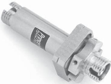
RFCX series Fiber Optic Rotary Adapters (FORAs) are unique since they have the identical cross sections and mounting features as their standard adapter counterparts, sometimes also called bulkheads or mating sleeves. FORAs allow the fiber to rotate freely while maintaining uninterrupted transmission of optical signal. Princetel's FORAs can be pop-in replacement of FC bulkheads.
