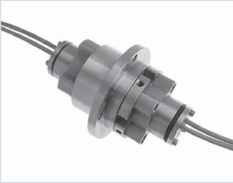
Dual-pass Fiber Optic Rotary Joints (FORJs) connect two independent fiber channels simultaneously. They allow uninterrupted transmission of optical signals while rotating along the common mechanical axis. The RJ2 series FORJs feature enhanced ruggedness. It is designed to accommodate at least one multimode fiber. The other channel can be either single or multimode fiber.
