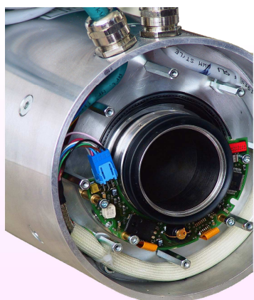
Integration of a SCS KIT 101 encoder inside a hollow shaft 145ST
