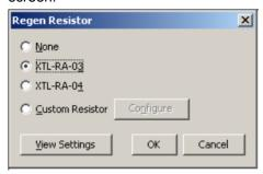
A.2.2.2 Select *Custom Resistor* and then click **Configure** to open the *Custom Regen Configuration* screen.
