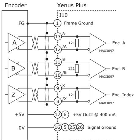
CONNECTIONS WITH NO INDEX SIGNAL
