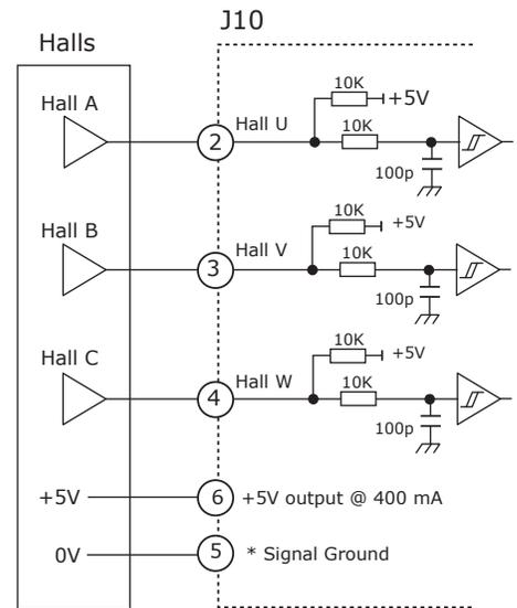
\* Alternate Sgnd connections on J10 are pins 16, 25, 26
