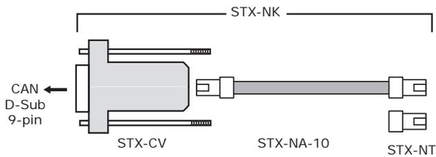
The connector kit for CAN networking (STX-NK) provides the parts to connect to a single drive. These comprise the adapter that converts the CAN D-Sub 9 connection to an RJ-45 type, a 10 ft (3m) modular cable, and a terminator that plug into an RJ-45 socket. The CAN address of the drive must between 1 and 127.
