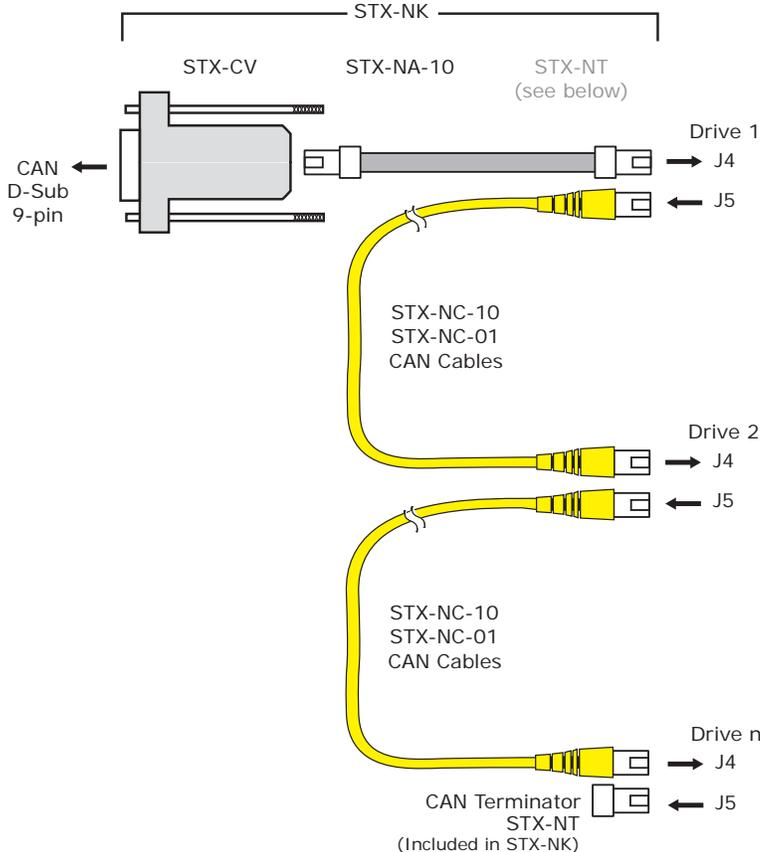
For multi-drive configurations over the CAN bus, the STX-NK is used in combination with CAN cables of the desired length. The network terminator is moved to the last drive in the chain and CAN cables daisy-chain from drive to drive to complete the signal path. Each drive must have a unique CAN node address between 1 and 127. CAN node address 0 is reserved for the CAN controller.
