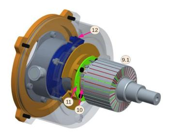
Figure 4 Sensor concept and the main motor rotor
