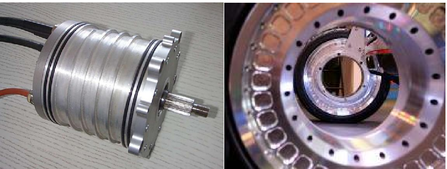
Left: housed motor with water cooling channels; right: hub, outer rotor motor
