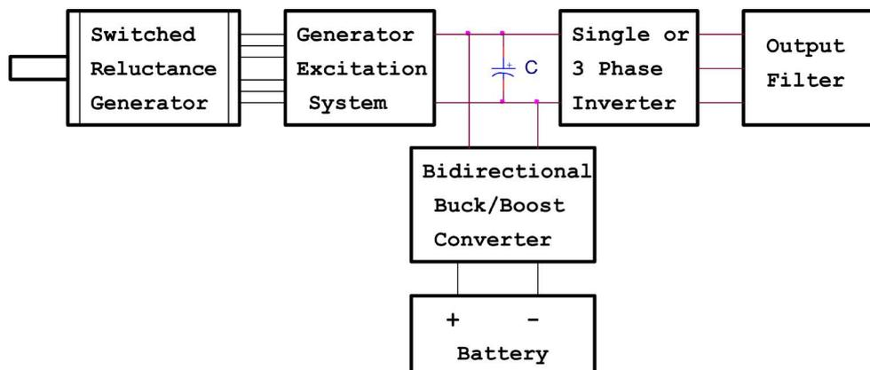
Figure 1. Functional block diagram of power conversion components in switched reluctance generator set
