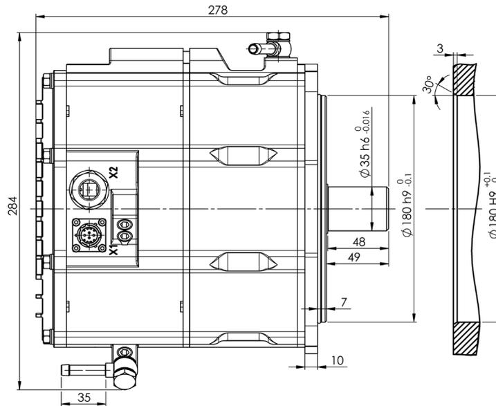
5kw generator dimension drawings
