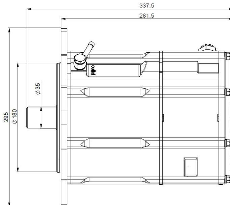
10kw generator dimension drawings
