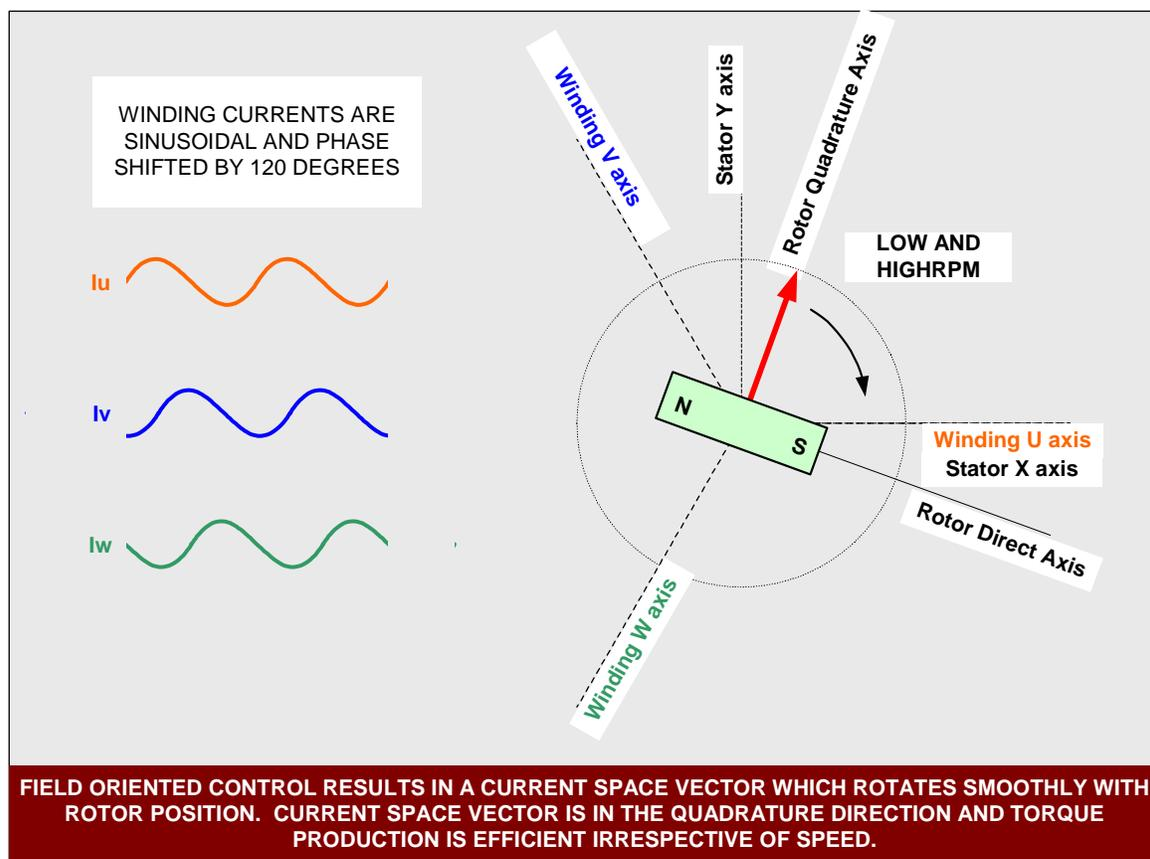
In Field Oriented Control, motor currents and voltages are manipulated in the d-q reference frame of the rotor. This means that measured motor currents must be mathematically transformed from the three-phase static reference frame of the stator windings to the two axis rotating d-q reference frame, prior to processing by the PI controllers. Similarly, the voltages to be applied to the motor are mathematically
