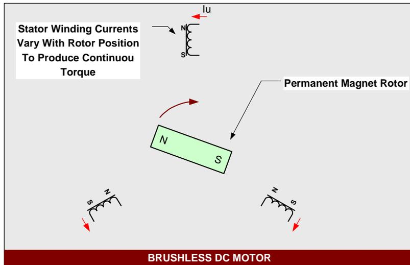
For the purposes of control system modeling and analysis, it is the convention to work in terms of winding currents rather than stator magnetic field. This is because motor currents are easily measured externally while fields (actually flux) are not.
