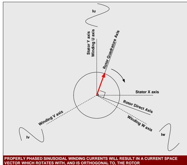
The sinusoidal winding currents should also be phased with respect to rotor angle so that the direct component of the stator current space vector is minimized (zero) and the quadrature component is maximized. This is the ideal case, and is achieved with varying degrees of success by different brushless motor control schemes.
